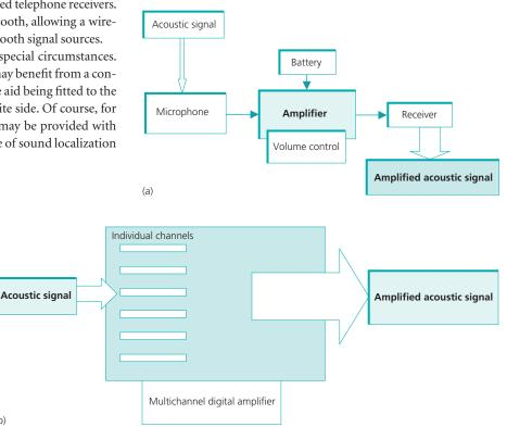
Figure 4.2 (a) Block diagram of a simple acoustic hearing aid. (b) Block diagram of a multichannel digital hearing aid.
