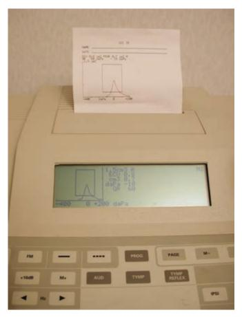
Figure 5.5 Impedence meter to measure middle ear pressures.
