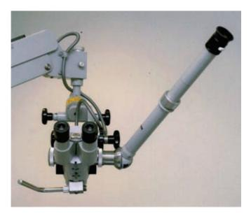
Figure 1.2 Binocular microscope with sidearm for observer.
